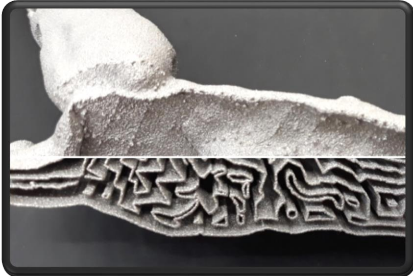
Removal of support structure
