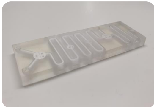
3D printed microchannel for unique chemical reactions
